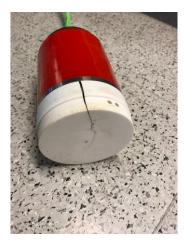
It is our professional judgement that the speed log sensor will perform better and more stable without the ice protecting plate because the ice protection plate itself may crack and cause the log sensor to fail.
